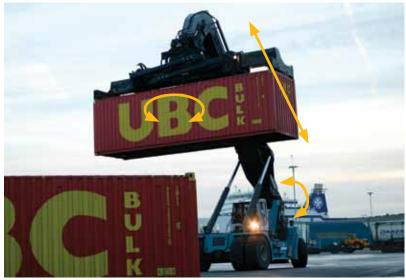
When rotating the container or lifting the boom with the container in a rotated position; there is some risk of damage to the boom or container. Adding a rotary sensor in the spreader slew ring will avoid any interference.
